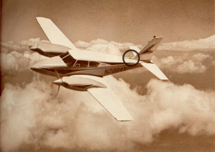
Flight shot shows rear-cabin air intake at forward base of new twin's vertical fin
