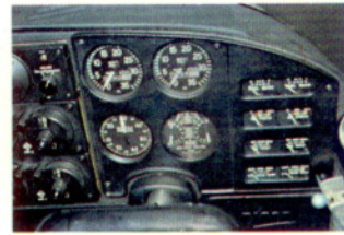
POWER INSTRUMENTS include separate tachometers to record individual engine hours, dual manifold pressure and fuel flow gauges.
