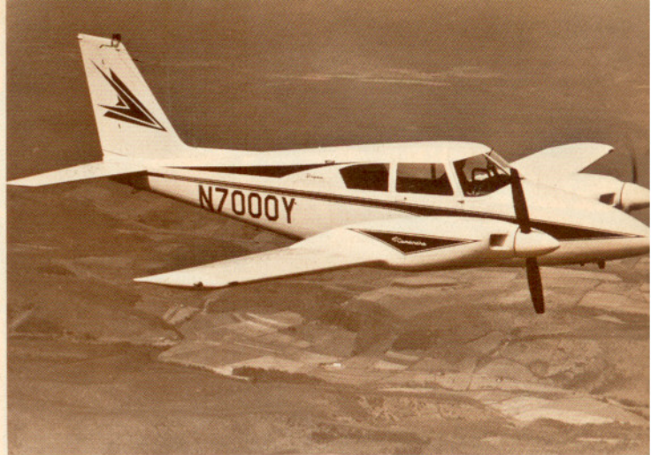
With one engine feathered, the Twin Comanche cruises 120-125 m.p.h. on other engine at normal cruise power. Yaw is so slight the plane is easily held with rudder pedal
