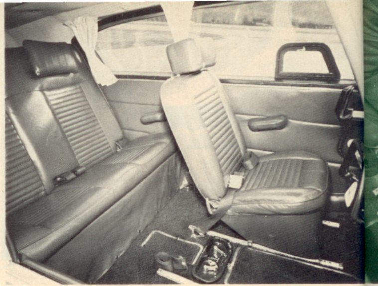
This is the Twin Comanche's Palm Beach leather-upholstered cabin, with right front seat removed. Fuel valves are in floor beside seat. Panel to rear of them is sump-draining system. In front is access hatch to emergency gear-extension system
